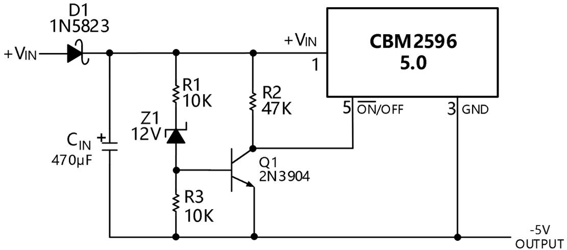
Figure 6. Undervoltage Lockout with Hysteresis for Inverting Regulator
