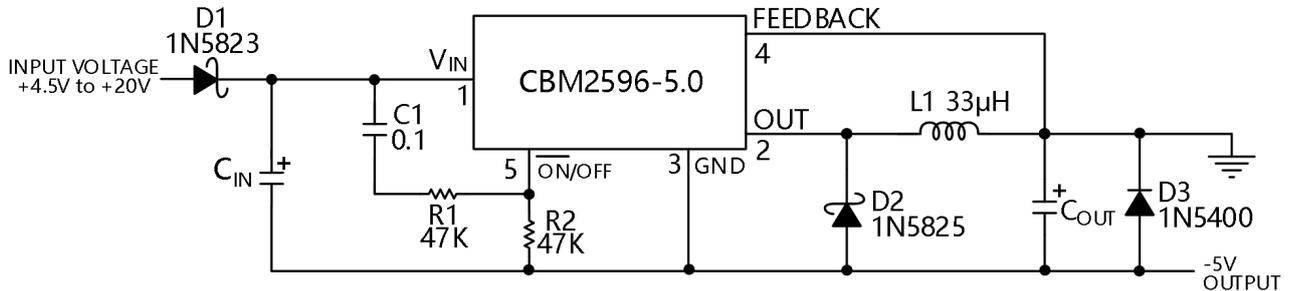
Figure 7. Inverting -5V Regulator with Delayed Startup
