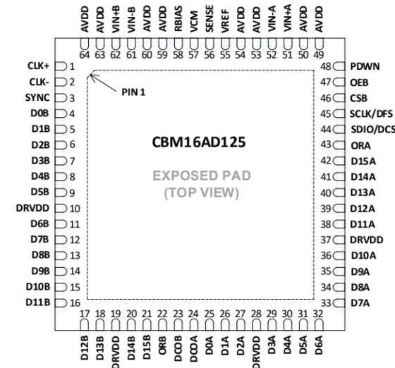
QFN Parallel CMOS Pin Configuration
