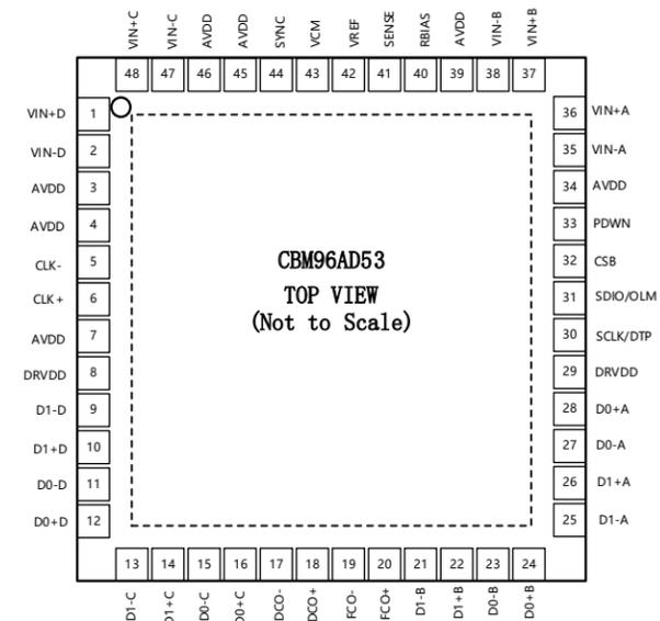
QFN-48 Pin Configuration, Top View
