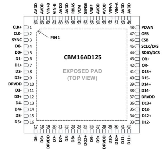
QFN Interleaved Parallel LVDS Pin Configuration
