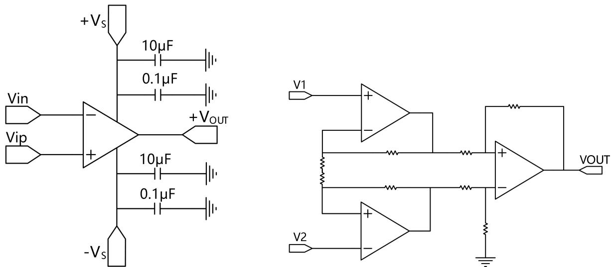
Figure 1. Amplifier with Bypass Capacitors
