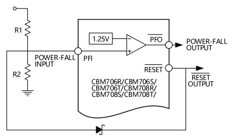
Figure 17. Power Fail Comparator
