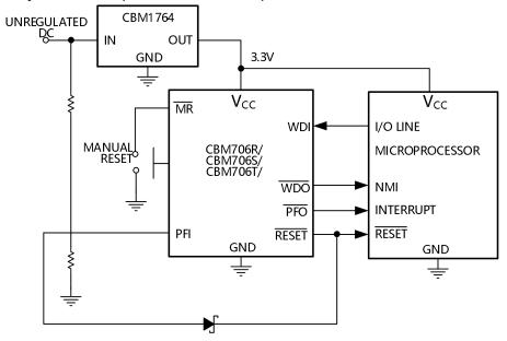
Figure 20. Typical Application Circuit
