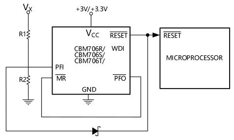
Figure 22. Monitoring 3 V/3.3 V and an Additional Supply V<sub>X</sub>
