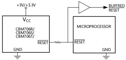
Figure 23. Bidirectional Input/Output RESET
