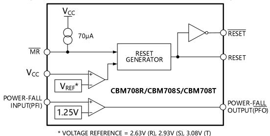
Figure 14. CBM708R/CBM708S/CBM708T Functional Block Diagram
