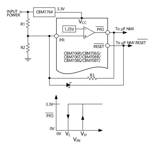
Figure 18. Adding Hysteresis to the Power Fail Comparator
