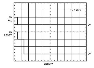
Figure 12. CBM706R/CBM706S/CBM706T and the CBM708R/CBM708S/CBM708T RESET Response
