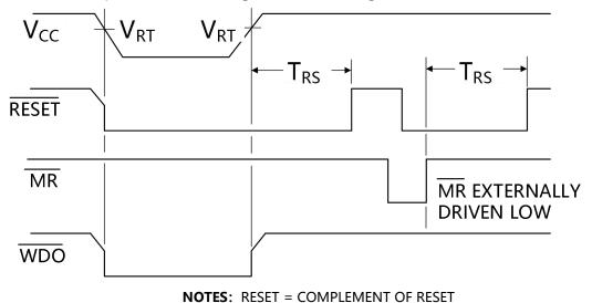
Figure 15. RESET, MR, and WDO Timing
