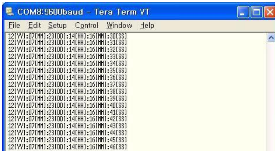
Fig6. CBM1363 RTC Data on Serial Terminal
