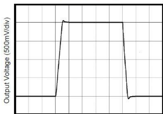
Non-Inverting Large-Signal Step Response
