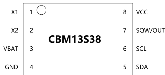
Figure 3. DFN8 Pin Configuration
